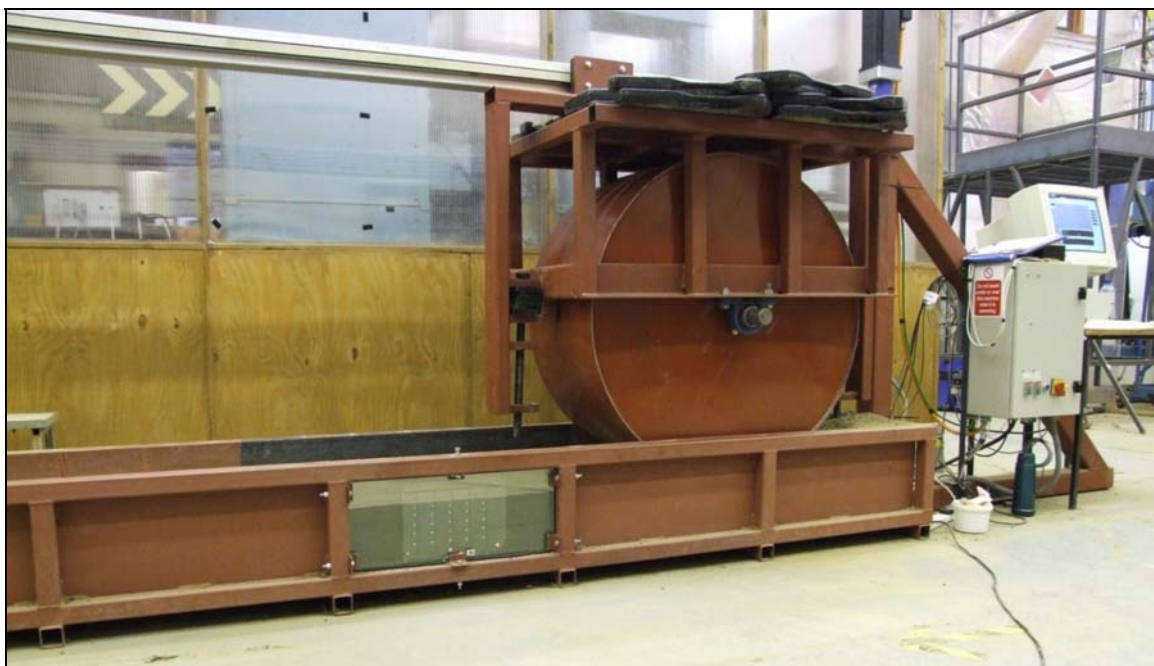
Figure 8 The Cranfield Cricket Rolling Simulator. In this configuration a 1 m diameter roller is rolling a 30% clay soil sample. Weights are added to the top of the roller which is towed and controlled by a computer. The tank can be removed and replaced with grass pitches too. The side window allows the deformation of the soil under the roller to be analysed with video processing software written at Cranfield University.
